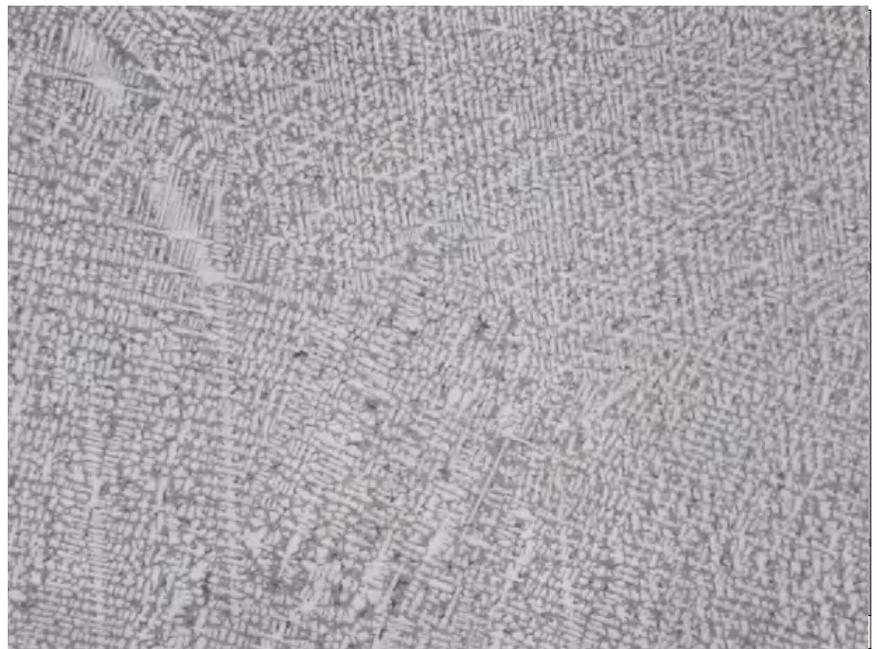
Optical Micrograph of a LION<sup>®</sup> 12 PTA Deposit at 500X.
