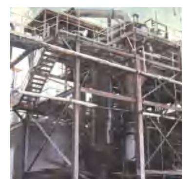
LIONG-30 alloy exhibits excellent resistance to commercial phosphoric acid. Its use is growing in the fertilizer industry for acid evaporators.
