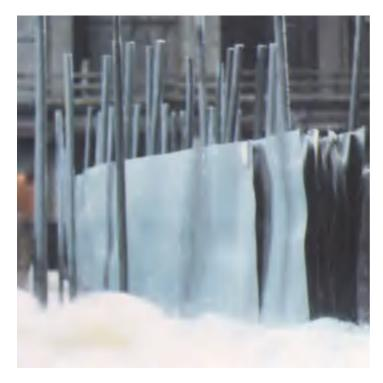
LION® G-30® alloy has outstanding resistance to hydrofluoric/nitric acid mixtures such as employed in the pickling of stainless steel. This particular operation involves aerated, 15% HNO<sub>3</sub> and 5% HF at 140 deg. F. (60 deg. C)
