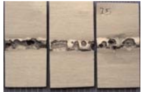
LION C-2000 alloy welded with matching filler metal.
